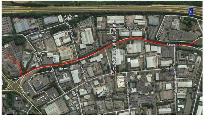
Figure 2-7 Proposed 33 kV cable route in red
