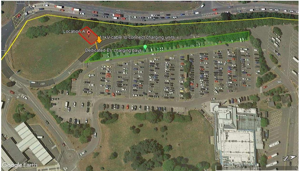
Figure 2-2 Detailed view of location A
