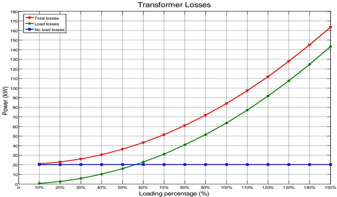
Figure 33: Losses of a 15 MVA transformer as function of loading
