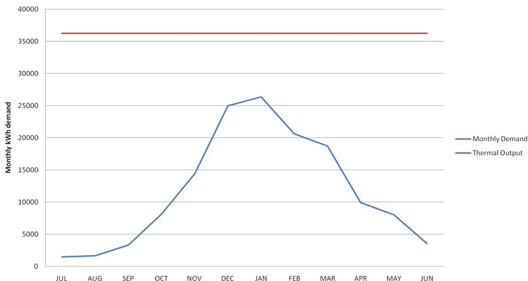
*Figure 21: Potential thermal output of GSHP vs. annual office heat demand at Hurst substation*
