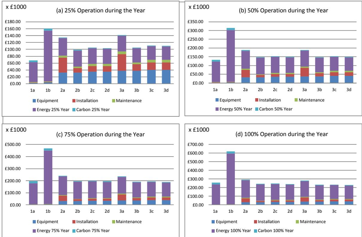
Figure 40: NPV of different heating system designs for increased transformer loading
